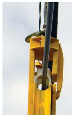
Cable Capture Prevents Pull Table Or Cable Jumping Edge
