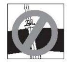
Sagging conduit creates "nodes" which can damage the hanger.
