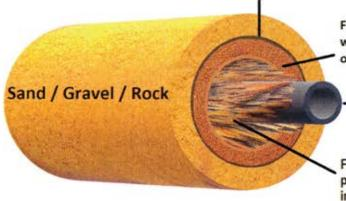
Fluid remains still around bore wall. This reduces fluid loss, wash out, and ground water infiltration.
